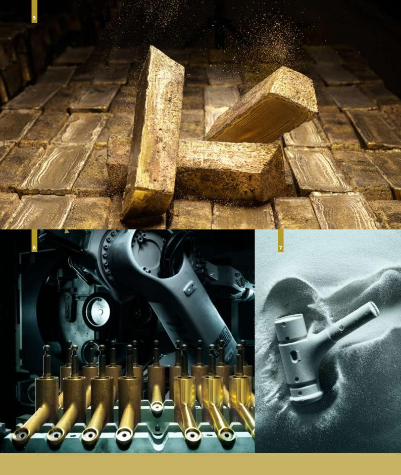
— To make the fittings, pure brass, which arrives in the form of ingots, is used. **6** — The basic shape of the fitting in brass. **7** — With low-pressure die casting, the brass is first melted and then poured into sand molds, creating the basic shape of the fitting in brass.
